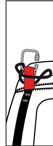
4 Close the mail- lon Rapide® by hand, then tighten using a set of pliers and making a 1/4 turn.
