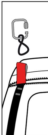
2 Push the bridle connecting point through the toric ring loop
