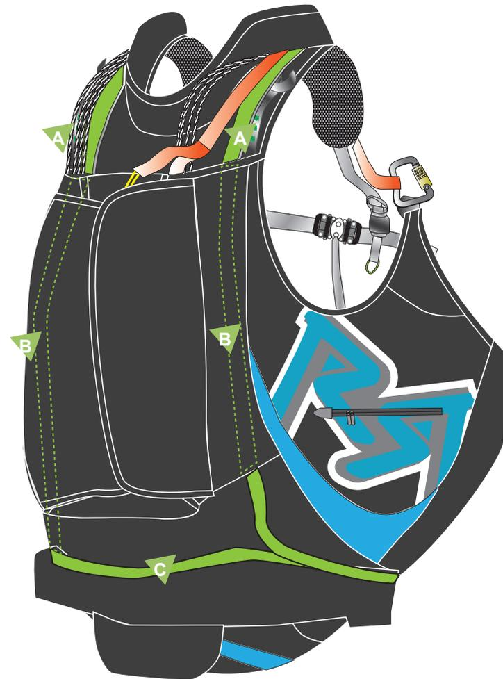
1. Place the Maillon Rapide® ( locking gate toward the top, facing outward ) and push it through the bridle loop under the flap. Place the O ring in the Maillon and twist it in a figure 8 configuration.
