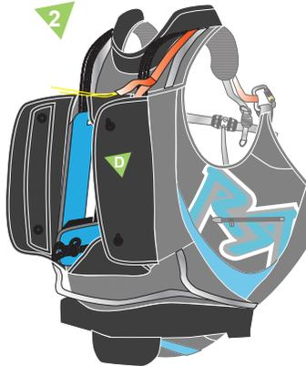
2. Fold the right flap, then, using a packing string, pull the small lines following the number sequence.
