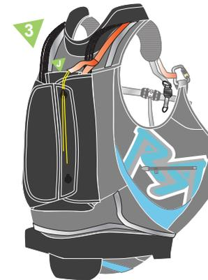
3. Push the two cables through the upper flap loop. Gently pull the string out.
