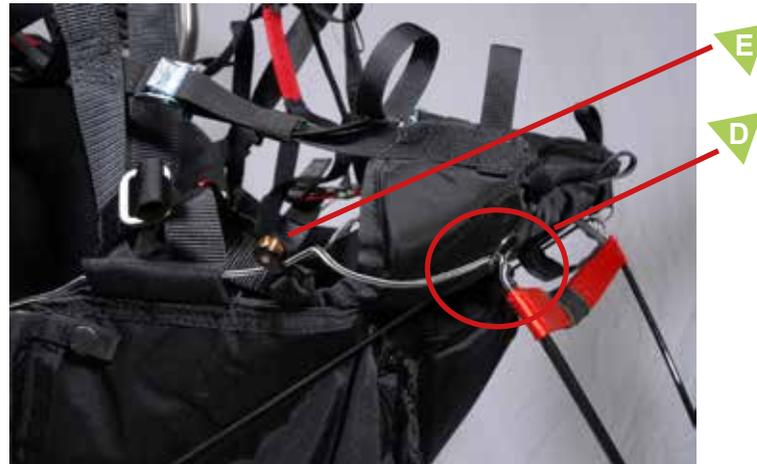
Push the accelerator cord and the elasticated line through ring "D".
