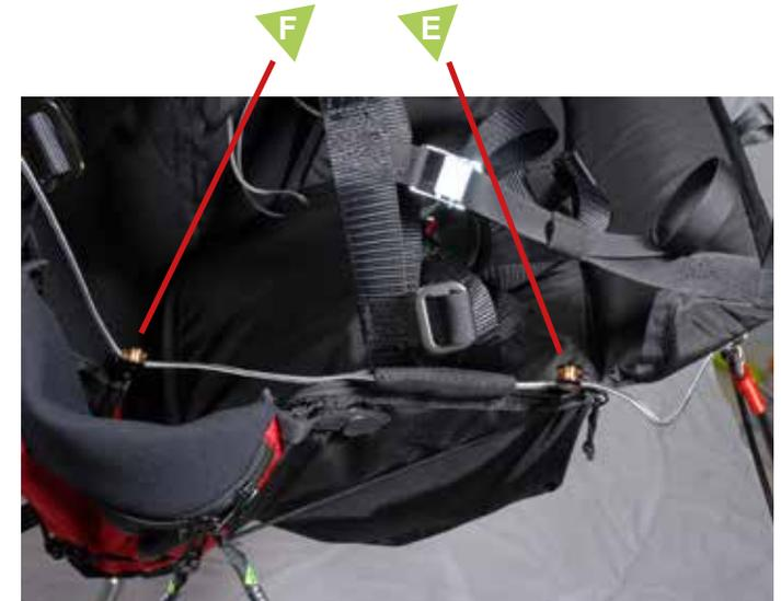
Push the cord through the Speed-bar pulley "E", then through pulley "F".
