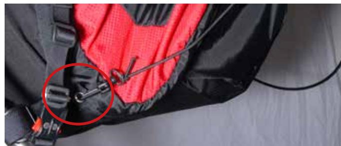
Insert the end of the cord through the paraglider riser split hook. Adjust the cord's length before tying a knot. Repeat procedure on the other side of the harness.
