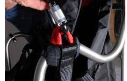
Fasten securely using the Velcros®, then push the glider's self-locking carabiner through to connect the wing's risers.
