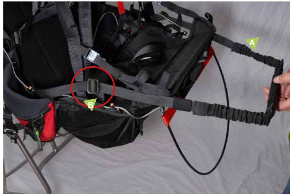
The PARAMOTOR EVO is pre-equipped to accept an accelerator ( Speed-Bar ).
