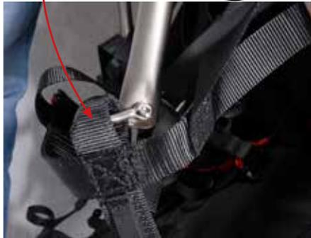
Fasten the bars ends to the harness loop straps using a shackle.
