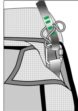
4 - Repeat the procedures 1, 2 and 3 with the other toric 8 shaped ring on the harness side. Tighten securely the Maillon Rapide® treaded gate - use a pair of pliers if necessary but do not tighten excessively.
