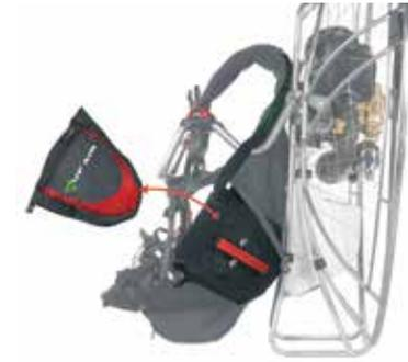
Installing the reserve parachute inside the container.
