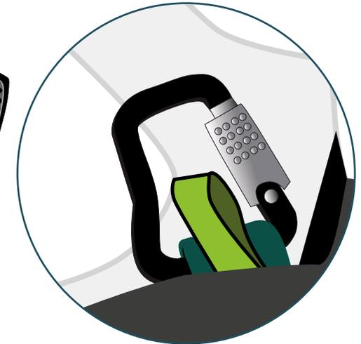
2 Push the loop through the ring located beneath the main location between the two straps
